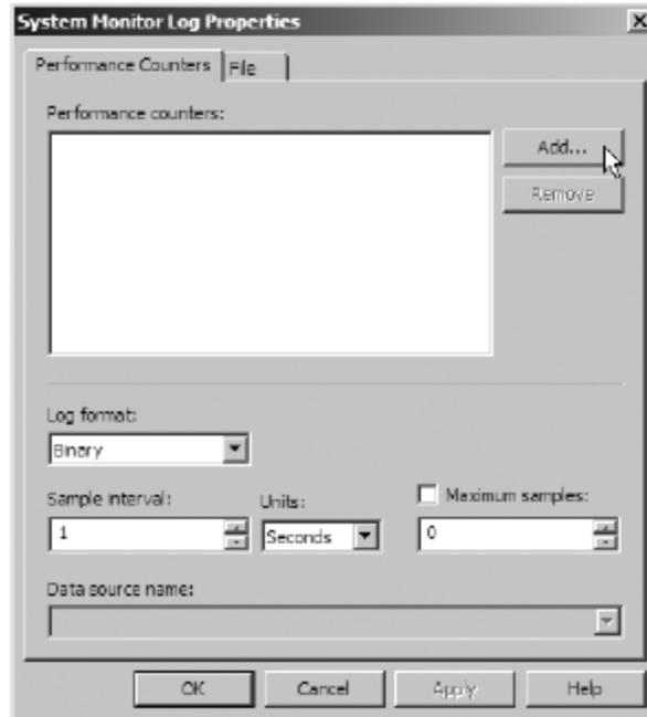
7. In the dialog box that appears, select <Local Computer> in the Select Counters From Computer drop-down list. Expand the Processor object from the Available Counters list. Select the % Processor Time counter and the \_Total instance. Note that you can click the Show Description box to find more information about the various parameters that are available. Click the Add button to add the counter to the Added Counters list.
